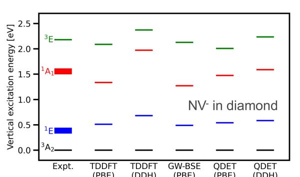
Unequivocal comparison of converged vertical excitation energies computed using TDDFT, **GW-BSE**, and **QDET**
